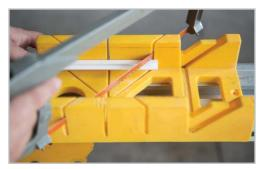
Mitre the two lengths of F-Rail at a 45 degree angle so they meet in the corner.
